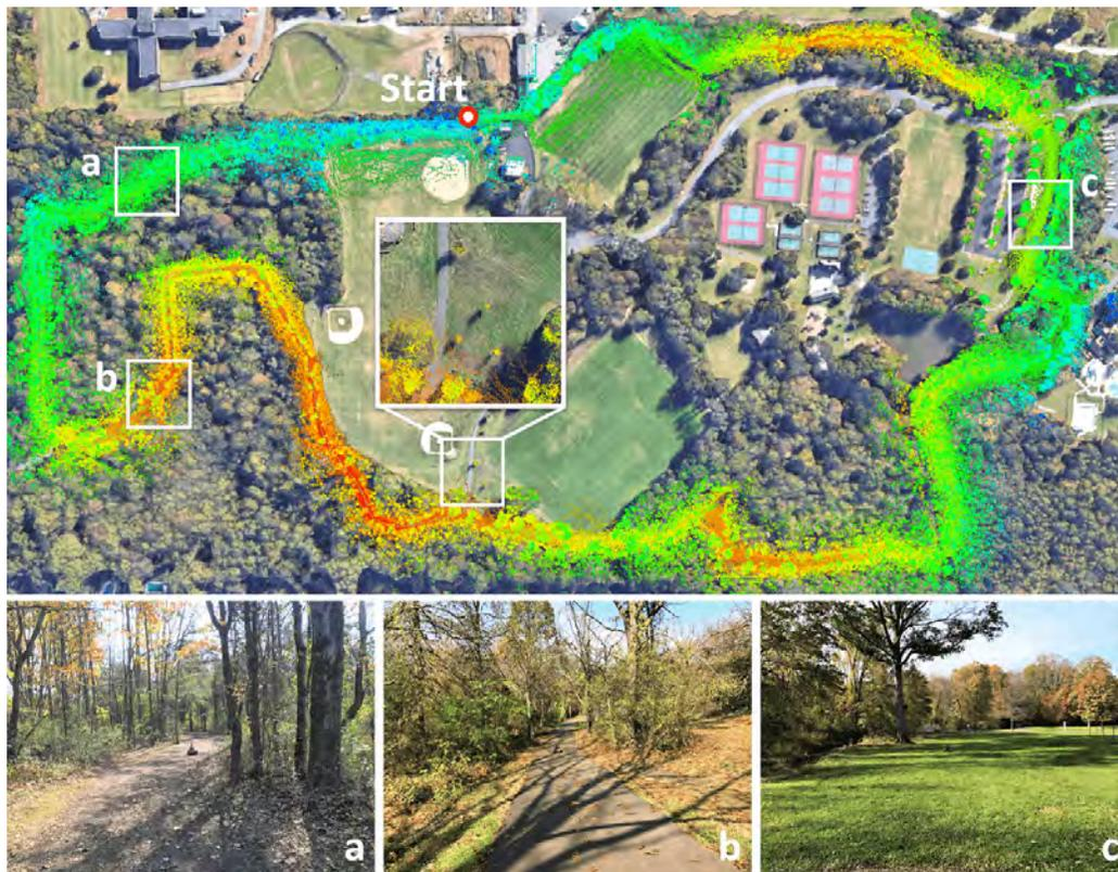
Figure 4.13: Experiment 3 LeGO-LOAM mapping result.
