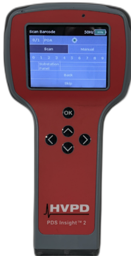
Figure 6.1: The Partial Discharge Sensor (PDS) Insight™ 2 from HVPD, which can record Transient Earth Voltage (TEV), Acoustic and High Frequency Current Transformer (HFCT) measurements. Using barcode stickers to identify the substation equipment of interest, measurements can be compared over time for diagnosis.
