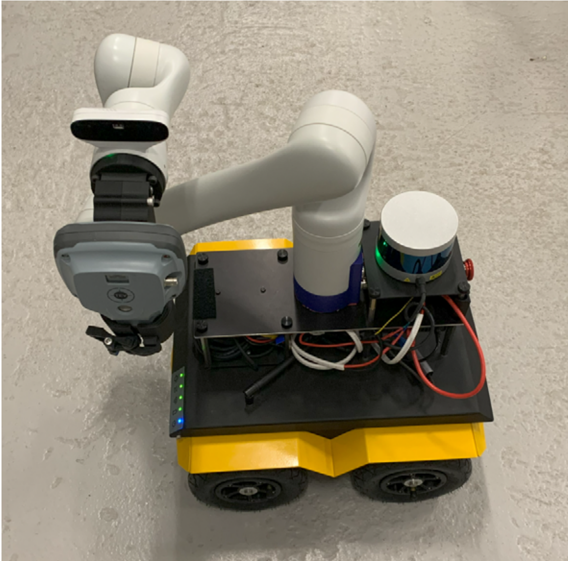
Figure 6.6: Complete hardware integration in travel configuration.
