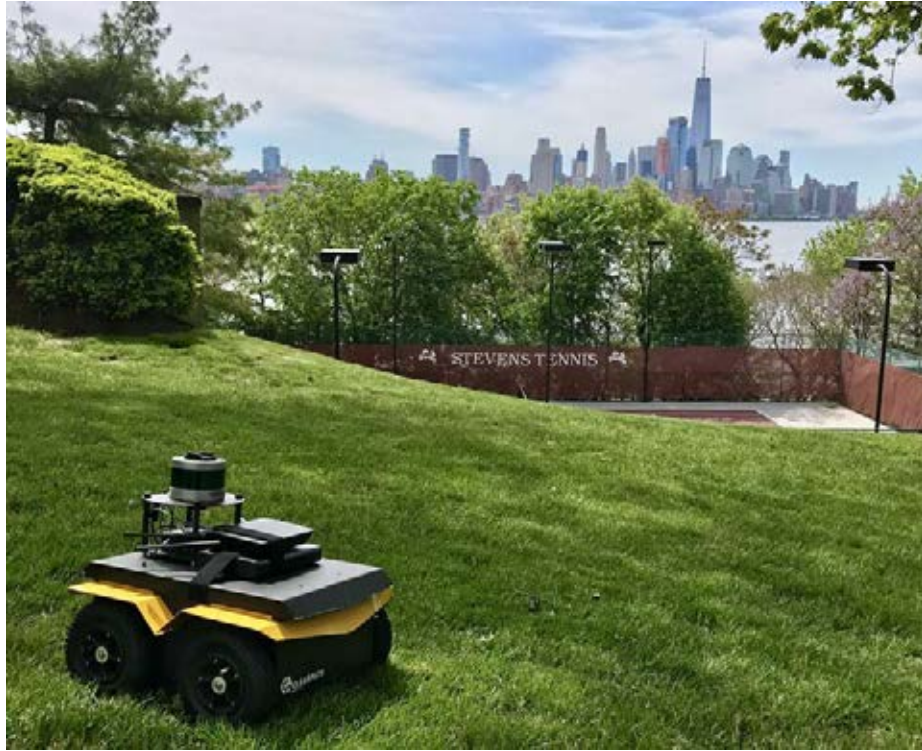
Figure 4.1: Unmanned Ground Vehicle from Clearpath Robotics called Jackal.
