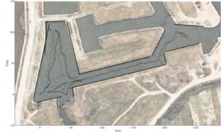
(b) The resulting map and trajectory from SLAM together with satellite image [3]
