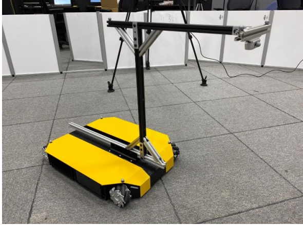
Fig. 4. Robot used for data collection, which features a downward facing camera and markers for recording pose using a motion capture system.
