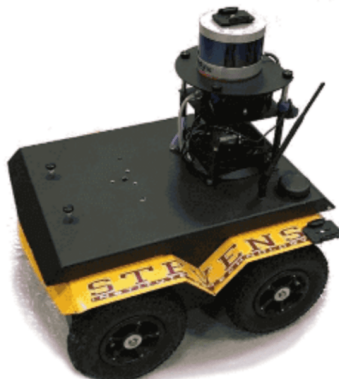
Figure 5.4: The Clearpath Jackal UGV used in our experiments.
