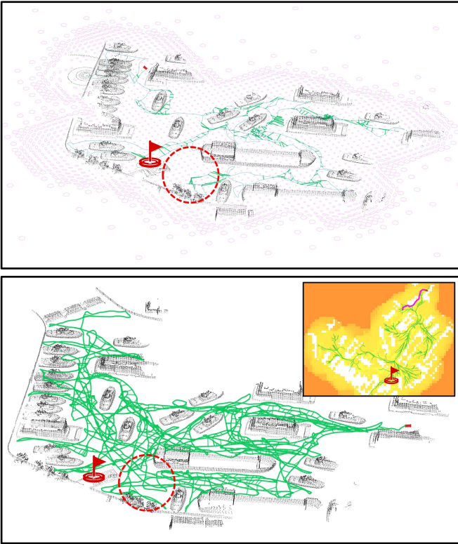
Fig. 5: Representative long-horizon exploration behavior in the 210\text{ m} \times 250\text{ m} basin sector. The top panel shows the exploration trajectory of VRVM-RRT, which exhibits denser recrossing and more redundant traversals before approaching the target coverage level. The bottom panel shows the corresponding result of VRVM-XIT, whose trajectory is more spatially organized and expands through the basin sector in a more directed manner; the inset further shows that the late-stage information field still provides coherent guidance for local proposal generation.
